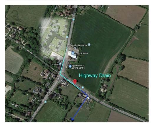
With a view to avoid digging up the A38 and laying new pipes that get us to this watercourse, we approached Gloucestershire Highways to gain permission to use their highways drain. This has been agreed subject to us making improvements to cracks and failures of their current pipes.
